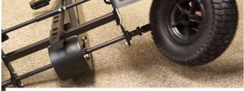
Wheel with star shaped hub attaches to the drive axle
