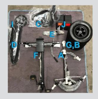
Install the rear fenders: Locate the two fenders and identify the left and right fenders by looking on the inside of the fenders and finding L for left and R for right.
