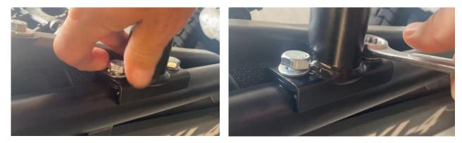
Install the end connection bolt and washer onto the end of the steering rod and tighten using a 13mm socket.
