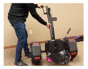
Remove all pre-assembled hardware: 2 bolt assemblies from the front axles (17mm socket), 1 bolt from the end of the steering shaft (13mm wrench), 1 screw from the front of the spoiler mount bracket (Philips screwdriver), and 1 bolt from the steering wheel mounting plate (13mm socket). Be careful to set and remember where each bolt belongs.
