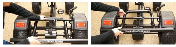
Replace the hardware with an Allen/hex wrench and a 13mm socket/wrench.
