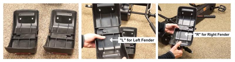
Install the fenders by sliding them over the fender support bracket as shown and lightly tap them on. You may need to move the hand brake lever to install the fenders fully.
