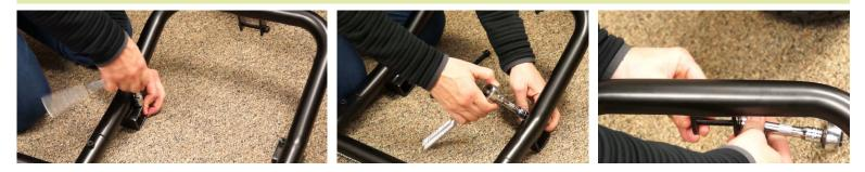
Slide the rear bumper frame metal tabs onto the square frame of the kart.
