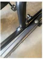
16. Remove the bolt from the end of the passenger grab handle and the bolt from the left steering shaft brace. Slide the grab handle assembly through the right bracing rod and into the end connection. Slide the other end onto left steering shaft brace.
