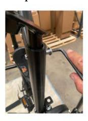
15. Line up the holes for the left bracing rod that is part of the steering shaft assembly, re-install the (2) bolts and washers and tighten using a 17mm wrench. Next, install the right bracing rod, re-install the hardware and tighten.
