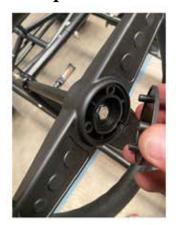
25. Install the spare tire mounting bracket to the front end assembly. It will thread into the mounting hub. Tighten by hand. Next, set the spare wheel hub over the bracket with the air fill facing down. Insert the spacer into the center hub facing down and thread the mounting bolt through the center. Tighten using a 17mm socket.
