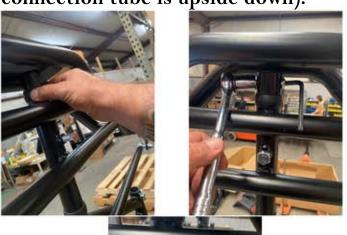
21. Connect the steering ball joint to the steering tab. Tighten using a 15mm open end wrench and a 19mm wrench
