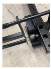
6. Re-install the (2) bolts and washers to connect the right and left brake assembly and tighten using 13mm wrenches. Be sure both ends of the brake rod are facing backwards.
