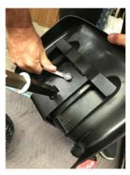
10. With the seat installed in the last position, stand the back end up so it's resting on the seat back (picture below shows seat frame before seats are installed) Next, locate (2) pedal sets. These will be marked L&R. The pedal marked L is installed on the left crank arm, R is installed on the right crank arm of EACH side. NOTE: the left pedals are left hand threads so they will screw into the crank arm counterclockwise. Tighten all 4 pedals using a 15mm open end wrench.
