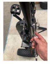
12. Remove hardware frm the front yoke Slide the front yoke over the (2) connector tubes. You may need to pull the rear assemblies together to install the yoke onto both tubes. Be sure that the spare tire mount is facing up.
