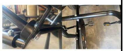
17. Tighten both sides of the rear assembly, (4) bolts and (4) nuts that were not tightened earlier
