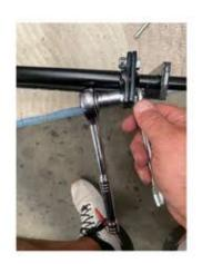
7. Remove the nut and washers from the parking brake cam and install in the hole on the left brace, just below the brake arm. In the resting position, the cam will be on top of the "J" hook Install so there is a white nylon washer on either side if the bracket, then a metal washer, then the lock nut. NOTE:Do NOT tighten the lock nut all the way. Tighten until the nut makes contact, then back off 1/2 turn. The brake cam should move up and down freely.
