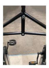
19. Loosen pivot stop bolt on the front assembly and slide the front assembly over the front connection tube. Make Sure the bolt is loose enough for the front assembly to slide all the way onto the connection tube.
