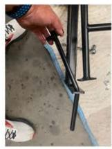
5. Remove the (2) nuts and washers and (2) bolts and washers fron the rear frame on both sides. Next, insert the hand brake through the support bracket of the rear assembly. Install the nuts and bolts connecting the rear frame connector to the right and left rear frame. DO NOT TIGHTEN
