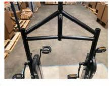
13. Remove steering bracing arm bolts from each side.
