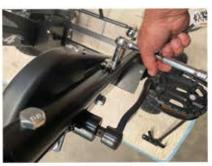
14. Install the end connection that is part of the left side steering shaft into the end of the yoke connector tube. Thread the bolt from the bottom side. Note that there are threads on the top side of the hole. Tighten using a 7mm Allen wrench. Once tight, install the washer and lock nut to the exposed threads and tighten with a 13mm wrench. Repeat procedure on the right side using the single end connection provided.
