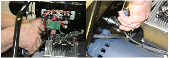
Only cut the plastic wire ties that secure the Power recepticle cable(s), including the ties that keep the black corregated plastic cover closed.
