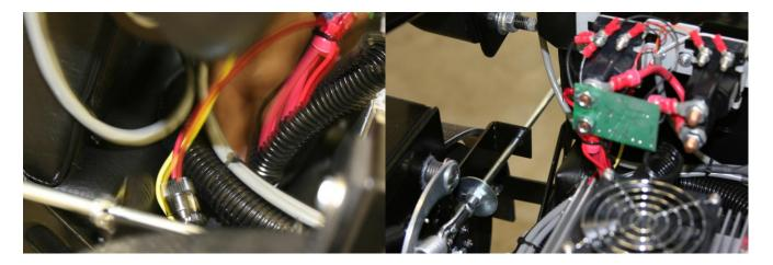
After the power recepticle wires are freed up, use the ½"wrench to CAREFULLY remove the nuts that secure the green circuit board. Afterwards, remove the nut that holds the metal loops that are attached to the <u>lower left post</u>.
