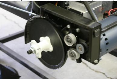
Next, remove the screws that hold the plastic cover that covers the wire connector posts.
