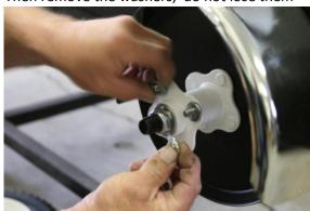
Remove the 5 screws that hold the side fender plate – note the screw that is under the fender.
