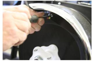
The fender plate is off – we will remove the plastic power recepticle later.
