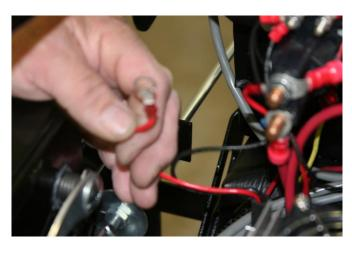
Then, use the 5/16" nut driver to remove the top left nut that secures the metal loops to that top left post.
