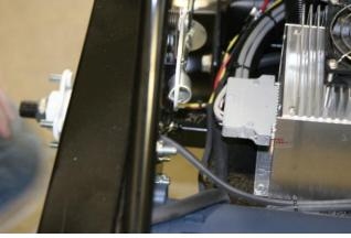
Slip off the black corregated plastic cover from the portion of the power recepticle cables/wires that go up to the wire connector posts. (There is a slit on the sideof the black corregated plastic cover) Then you may continue snipping the remaining 2 plastic wire ties that go up to the wire connector posts.
