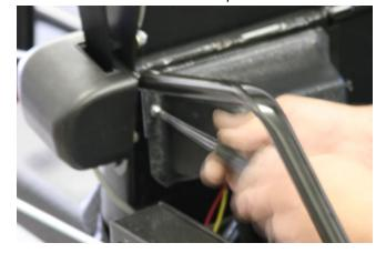
Use the wire snips to clip the plastic wire ties that secure the power recepticle cord wire(s).
