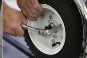
Use the 3/4" Ratchet Socket Wrench to remove 4 nuts
