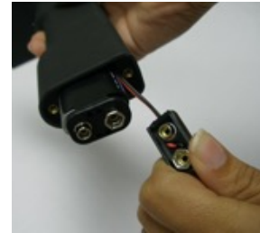
Disconnect battery snap, remove battery clip
