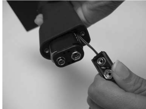
Figure 4 Disconnect battery snap, remove battery clip
