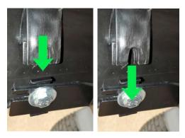
The inside plastic slot must fit between the washer and the frame metal support bracket. Tighten the bolts using a 13mm socket/wrench, so the spoiler stays securely. Be careful not to crack the plastic by over-tightening. Finish tightening the Philips head screw in front to secure the spoiler.
