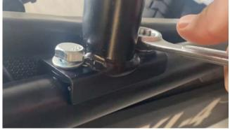
Install the end connection bolt and washer onto the end of the steering rod and tighten using a 13mm socket.
