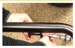
Slide the rear bumper frame metal tabs onto the square frame of the kart.
