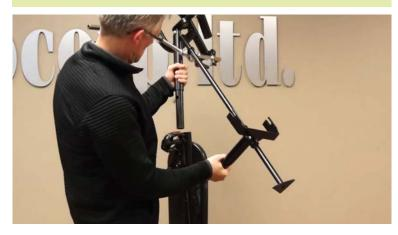
Use a 17mm socket or wrench to replace the 2 bolts/washers by the chain drive on the rear assembly to attach the steering column brace. Do not tighten the front bolt all the way yet. This maneuverability is needed to shift and position the steering rod next.
