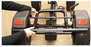
Replace the hardware with an Allen/hex wrench and a 13mm socket/wrench.
