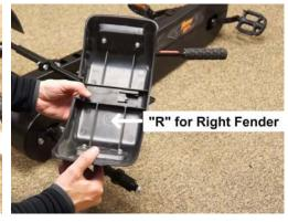
Install the fenders by sliding them over the fender support bracket as shown and lightly tap them on. You may need to move the hand brake lever to install the fenders fully.
