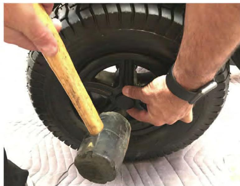
Install both front wheels and tighten using a 17mm socket. The valve stems should face inward while installing the wheels
