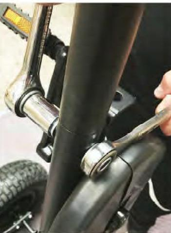
Install the washer and lock nut onto the bracing rod threaded end and tighten using a 19mm wrench or socket.
