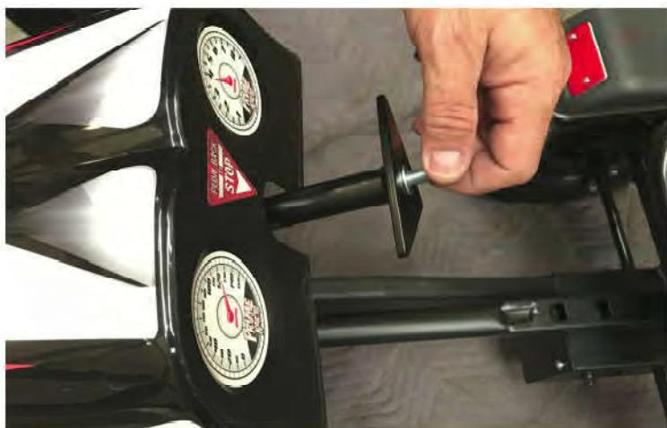
Slide the steering wheel over the plate, then slide the bolt and washer through the steering wheel and tighten using a 13mm socket.
