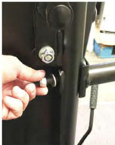
Install both front wheels and tighten using a 17mm socket. The valve stems should face inward while installing the wheels
