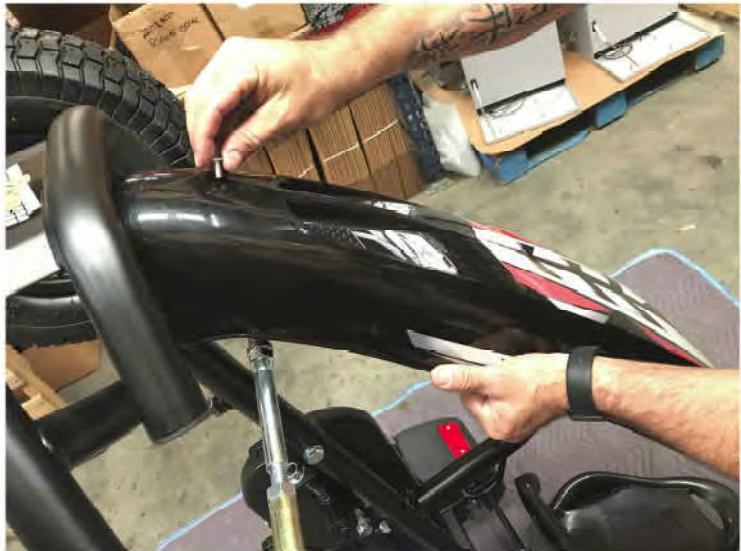
Now place the plastic top of the spoiler over the metal support brackets as shown below, then slide the metal clips (C) onto the metal brackets where the spoiler sits, then position it with the washer on the outside towards the locking nut and tighten using a 13 mm wrench or socket.
