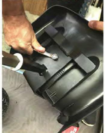
Slide the metal seat frame into the slot on the back of the plastic seat and line up the hole on the seat frame with the hole on the seat.
