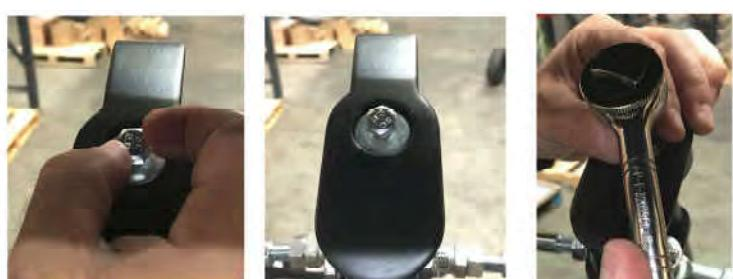
Install the frame connection bolt, washers and nut. Tighten using a 19mm wrenches and socket.
