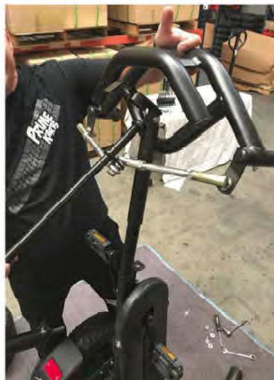
Slide the front assembly into the tube of the rear assembly
