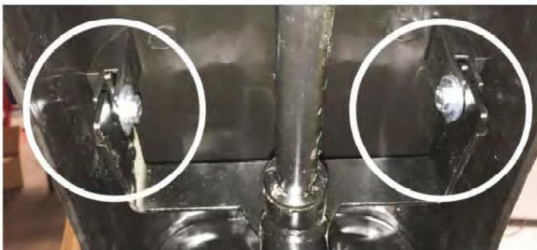
After the bolts are tight on the top of the spoiler mount, you can tighten the screw at the bottom of the spoiler using a Phillips screwdriver.
