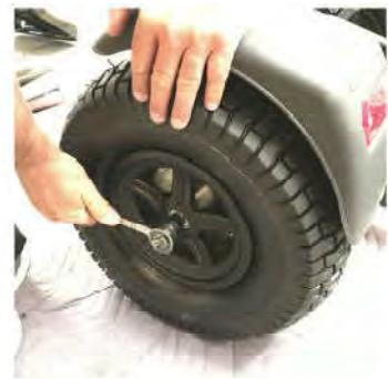
Using a 17mm socket, remove the bolt and washer from the coast side of the rear axle. Slide the coast wheel on the axle with the air fill valve facing INWARD.
