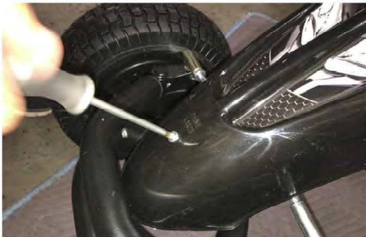
Now back out the existing bolt in the steering wheel metal plate.
