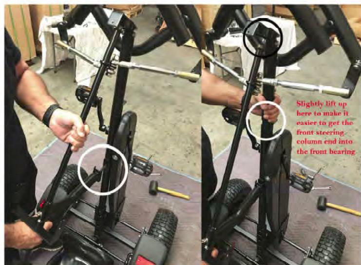
Install the end connection bolt and washer onto the end of the steering rod and tighten using a 13mm socket.
