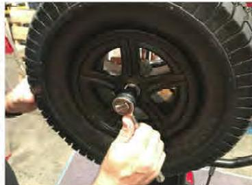
Install the Phillips head screw through the hole at the bottom of the spoiler into the metal tab on the kart
