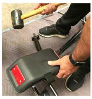
Install the fenders by sliding them over the fender support bracket as shown and lightly tap them with a rubber mallet. You may need to move the hand brake lever tab to fully install the right side fender.
