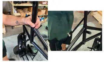
Install the washer and lock nut onto the bracing rod threaded end and tighten using a 19mm wrench or socket.
