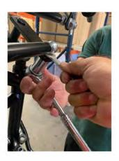
Install the steering wheels and tighten using a 13mm socket. Once tight, attach the steering wheel cap with a rubber hammer.
