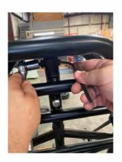
Install the steering linkage to the bottom of the left side steering shaft. The lock nut will be on the top side. Tighten using a 13mm and a 19mm wrench.
