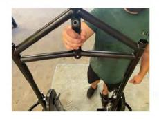
Install the steering shafts. The left steering shaft turns. The right is fixed. The front bolt threads into the bottom tube. Install the washer and lock nut and tighten with a 15mm wrench.
