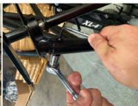
Line up the steering bracing rod brackets with the frame. Install the washers and nuts and tighten using a 15mm wrench.
