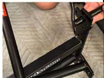
Slide the left side handbrake arm through the left fender support and line up rear connection bracket bottom holes with the two studs on the bottom. Install flat washers nuts and two bolts in the top holes with flat and lock washers. Tighten using a 13mm wrench. Repeat on the right side.
