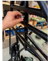
Install front end connection to the end of the connection tube. Install bolt and nut and tighten using a 15mm wrench.
