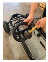
Install spare tire mounting bracket. It simply screws into the frame. Attach the spare tire using the bolt and tighten using a 17mm socket.
