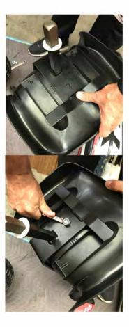
Slide the metal seat frame into the slot on the back of the plastic seat and line up the hole on the seat frame with the hole on the seat.
